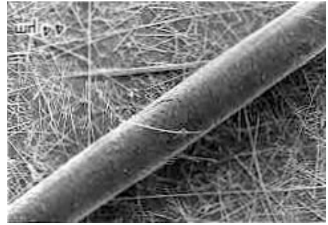
Amosite or brown asbestos
